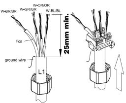
Step 1: Strip the cable for minimum 25 mm,pull the foll or braided shield back over the jacket.
