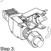
Insert the slotted screwdriver into the slot and rotate to open the wiring Management.
