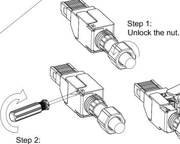
Insert the slotted screwdriver into the slot and rotate to open the jaws
